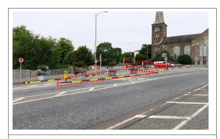
Node 2.2. N72/ Pole and street light should be removed/re-located. Hedge on right should be reduced to 3m over road level to a depth of 2.5m
