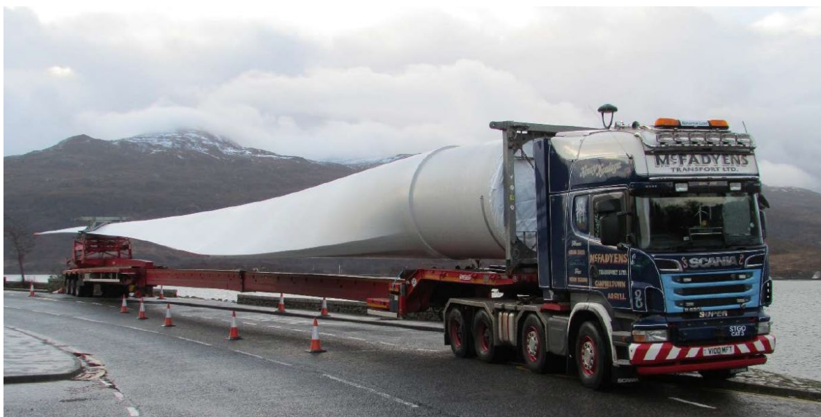
Plate 13-10: ‘Superwing’ Blade Carrier
