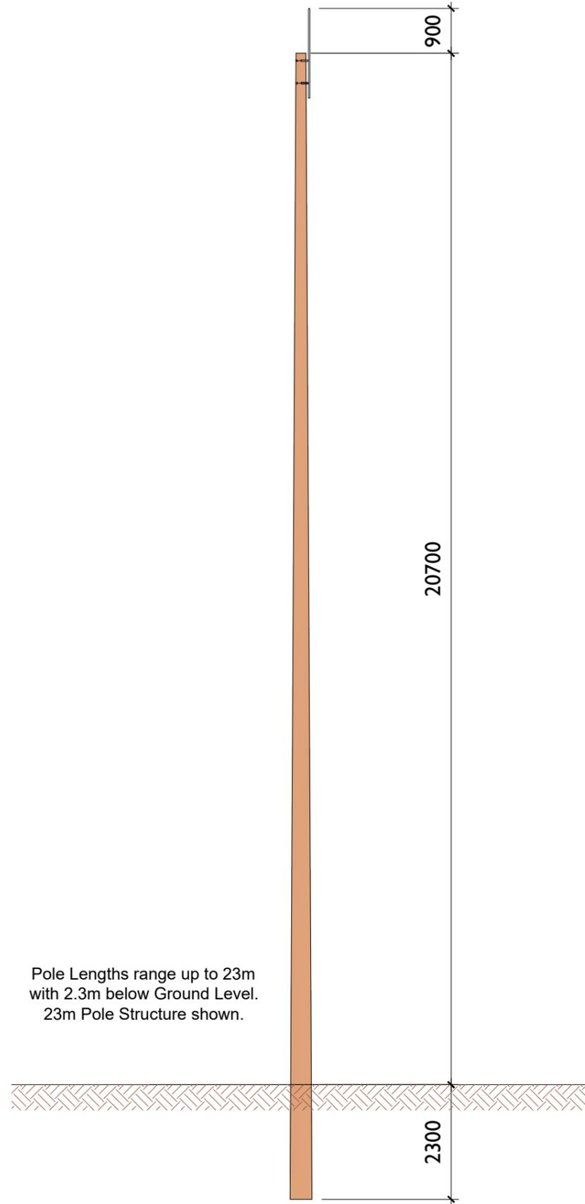
Pole Lengths range up to 23m with 2.3m below Ground Level. 23m Pole Structure shown.
