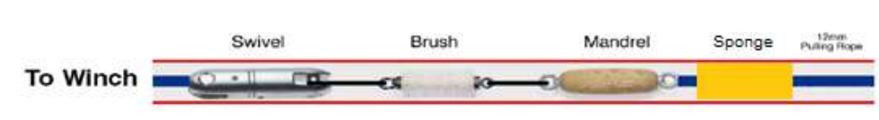
Figure 1 - Set up for Swivel, Brush, Mandrel and Sponge for Duct Proving and Cleaning
