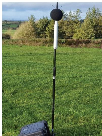
Image: Typical noise monitor unit as used during the recent project background noise monitoring campaign.
