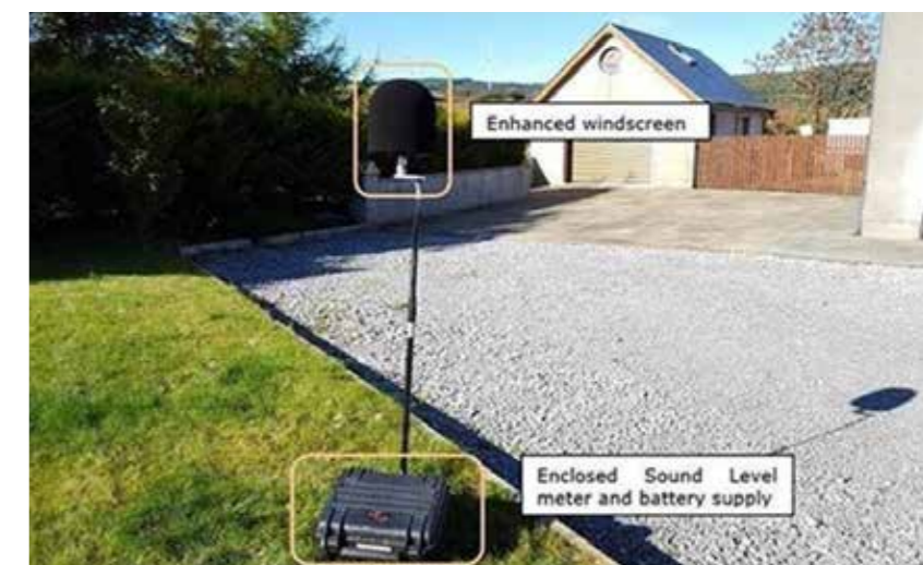
Typical noise monitor used to measure background noise levels during the design process
