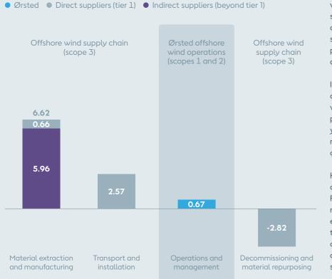
the total lifecycle emissions of an Ørsted offshore wind farm. This is primarily due to the carbon-intensive processes needed to manufacture materials for wind turbines and foundations as well as the fossil fuels used by vessels supporting the installation of our farms.
