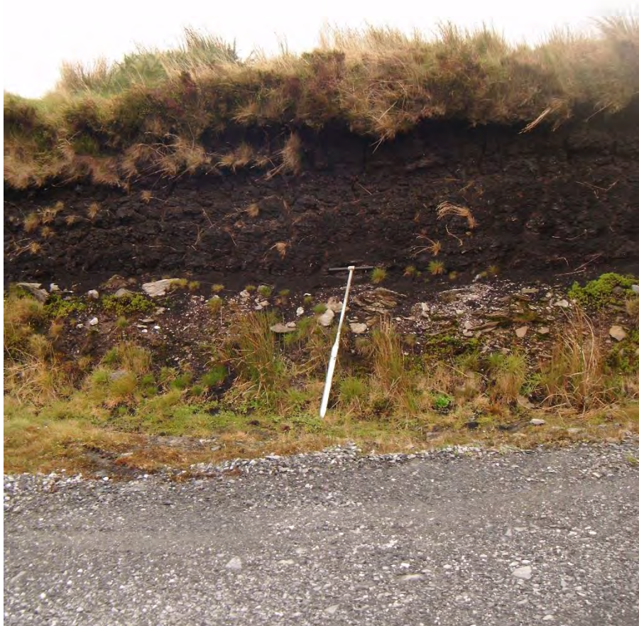
Figure 4: Exposure of peat overlying glacial till on the western margin of Area A. The till consists of clasts of crystalline rock in a dense silty-clay matrix. The abundance of cobble sized clasts has prevented substrate sampling during probing (reflected by refusal)
