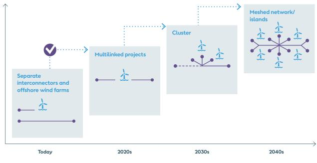
These cost-efficiencies can be even greater, if multilinked offshore wind farms are combined with optimised localisation of future power-to-X plants, as this leads to substantial system benefits and reduced transmission needs. Together, the required interconnector in 2050 can be reduced by 20%, compared to a scenario without multilinked wind farms and without redistribution of power-to-X products, the study suggests.
