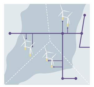
**Multilinked approach:** Offshore grid and wind farms planned and built together, combining export cables and interconnectors to multilinked offshore wind farms.
