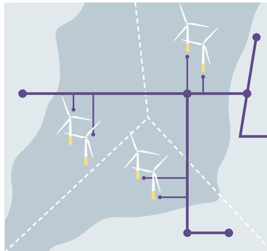
**Multilinked approach:** Offshore grid and wind farms planned and built together, combining export cables and interconnectors to multilinked offshore wind farms.
