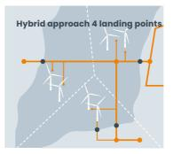
Offshore grid and wind farms planned and built together, combining export cables and interconnectors to multilinked offshore wind farms
