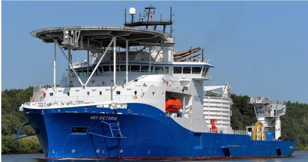
Photo 2.1. Specialist vessel for laying subsea cables – Cable Laying Vessel [Source: www.nkt.com ]
