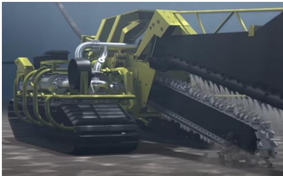
Photo 2.5. Exemplary tools for the mechanical cable burial [Source: www.boskalis.com ]
