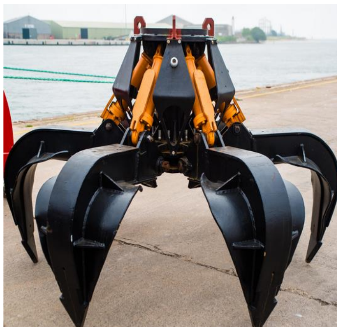
Photo 2.3. Exemplary grab for transferring boulders over the seabed area [Source: www.utrov.com]
