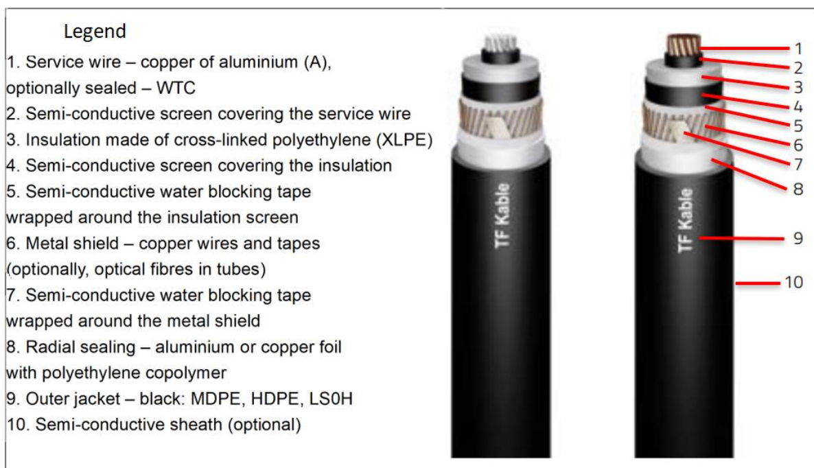
Figure 2.9. Construction of a cable intended for laying in an onshore cable bed area [Source: TF Telefonika catalogue]
