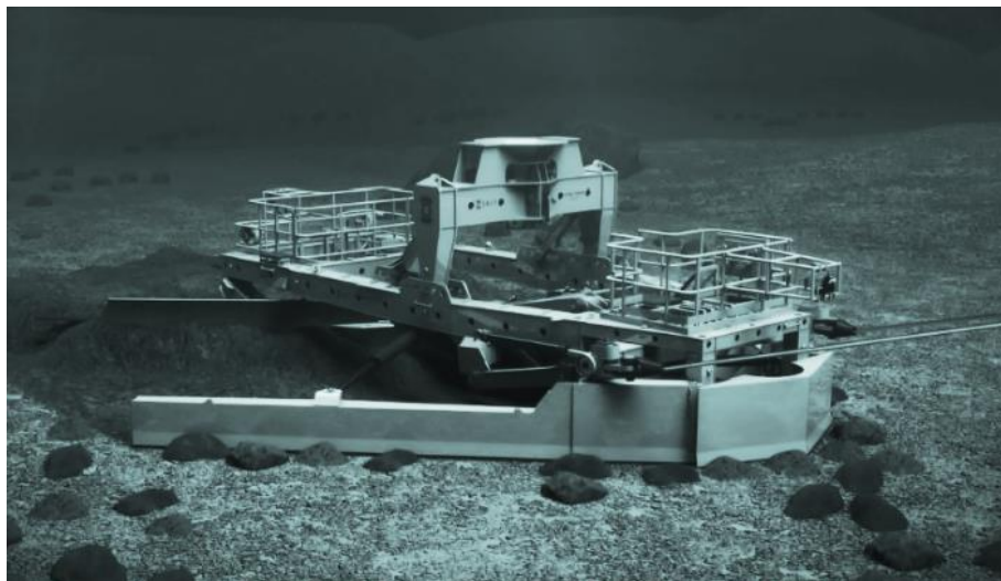
Photo 2.2. Exemplary plough used for clearing the seabed from boulders [Source: https://globaloffshore.co.uk/vessels-trenching-assets/pre-lay-plough/ ]
