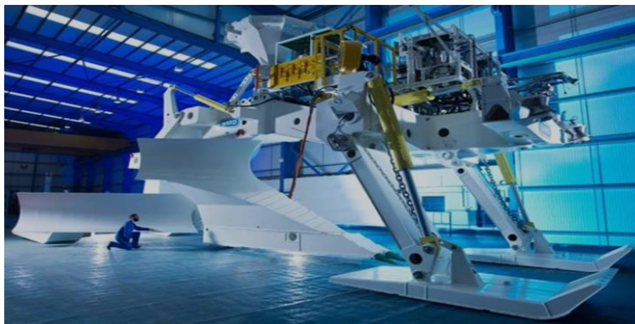
Photo 2.6. Exemplary submarine cable plough [Source: https://www.youtube.com/watch?v=wb1le4zRA2M ]
