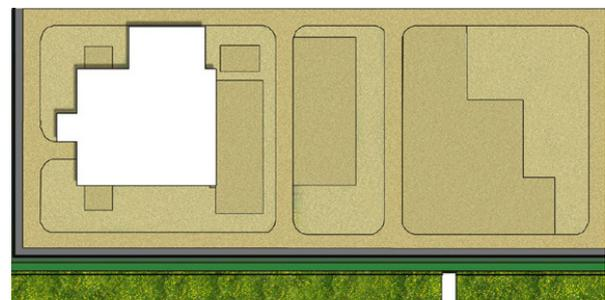
Road and Footings - Concrete with exposed aggregate. Elsewhere - Self binding gravel
