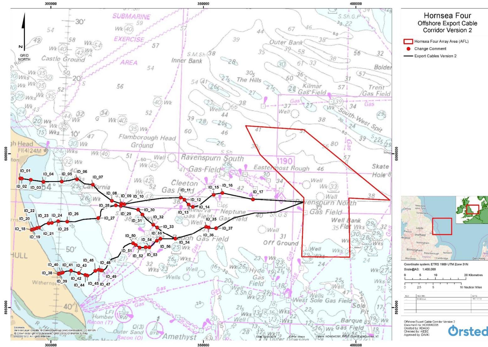
Figure 7. Hornsea Four Offshore Export Cable Corridor Version 2.
