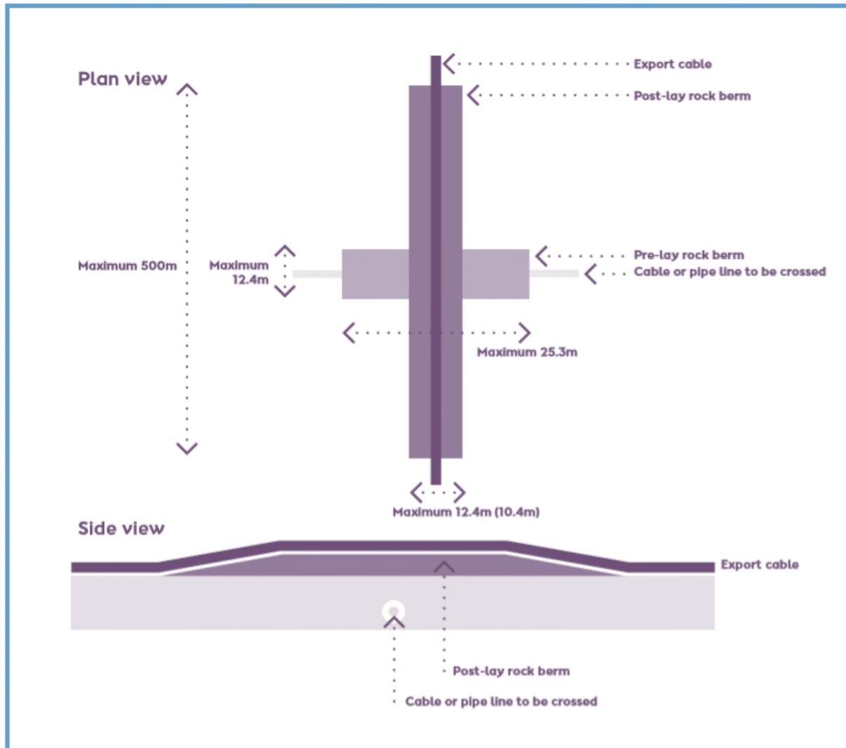
Figure 4.11: Offshore Cable Crossing (indicative only).
