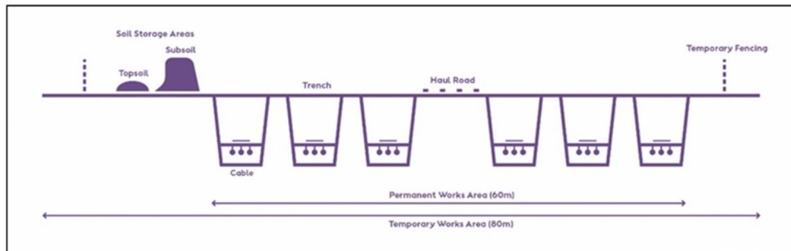
**Figure 4.18: Onshore export cable corridor indicative layout showing the maximum of 6 onshore circuits (indicative only).**
