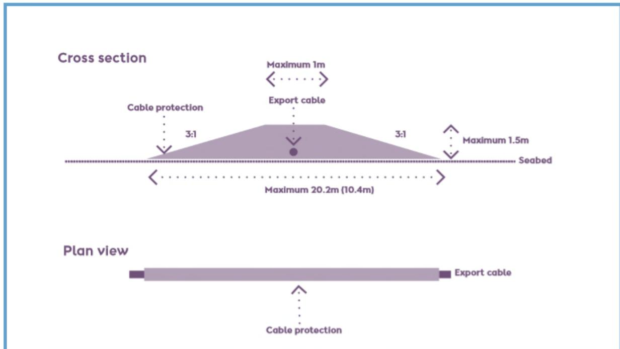
Figure 4.10: Cable protection via rock placement (indicative only).
