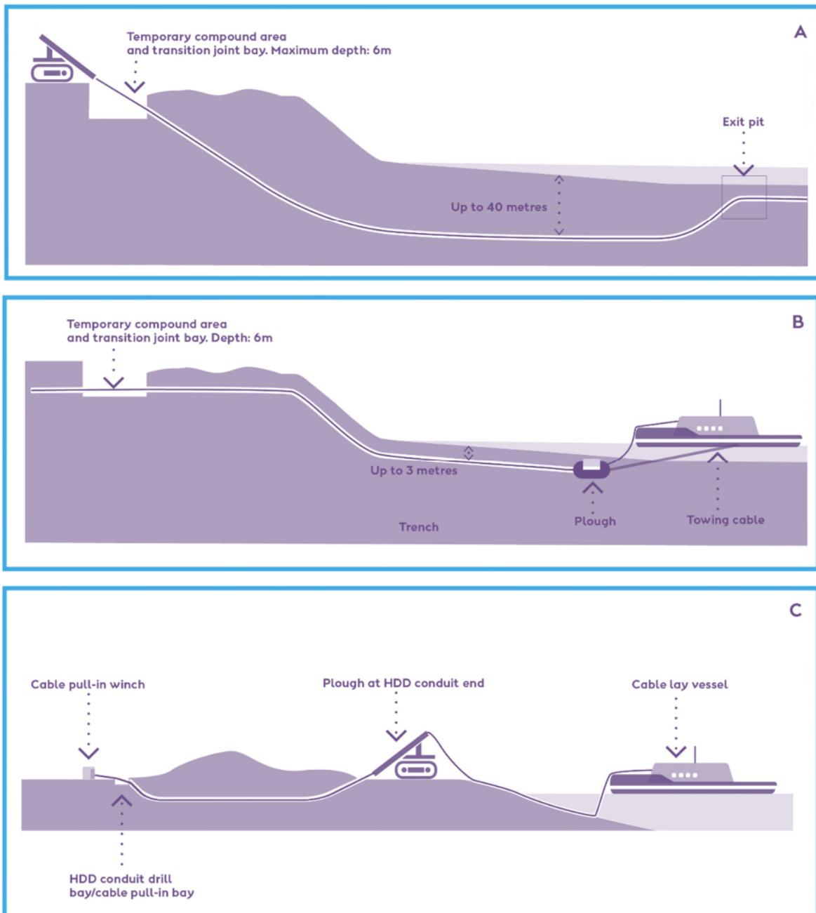
Figure 4.14: Indicative HDD and open cut arrangement (indicative only).
