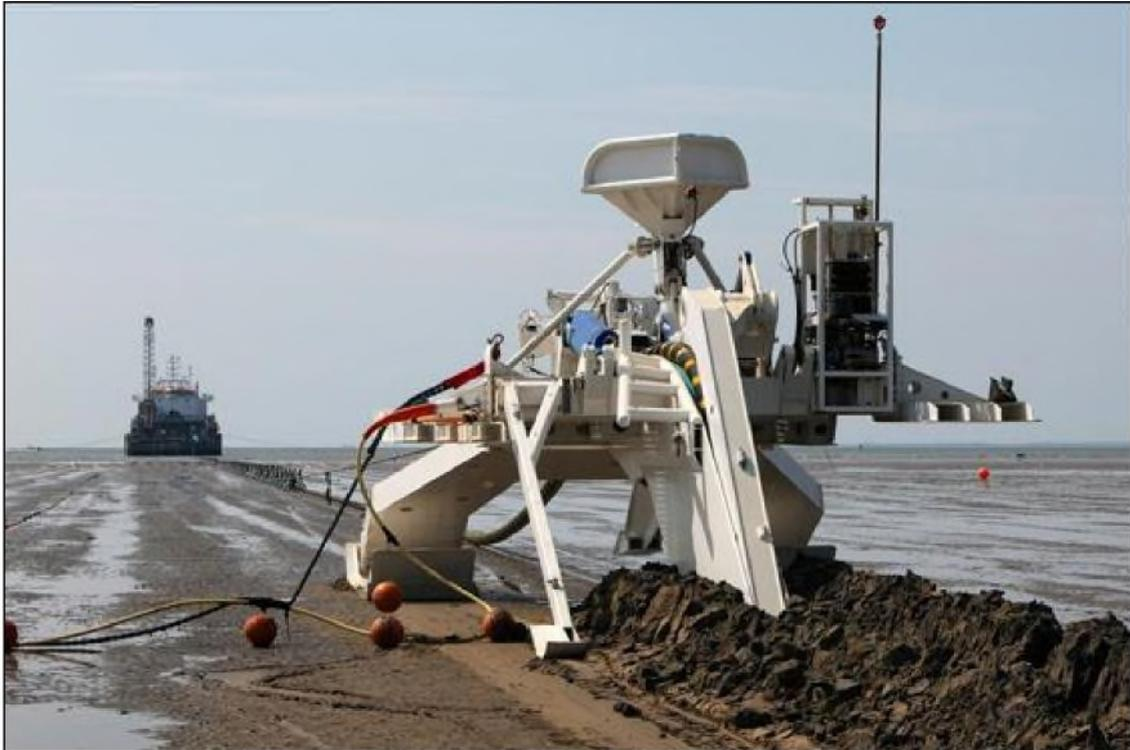
**Figure 4.16: Example of a cable plough pulled from an installation vessel. source: <http://www.4coffshore.com/s/about/equipmentTypes.aspx>.**
