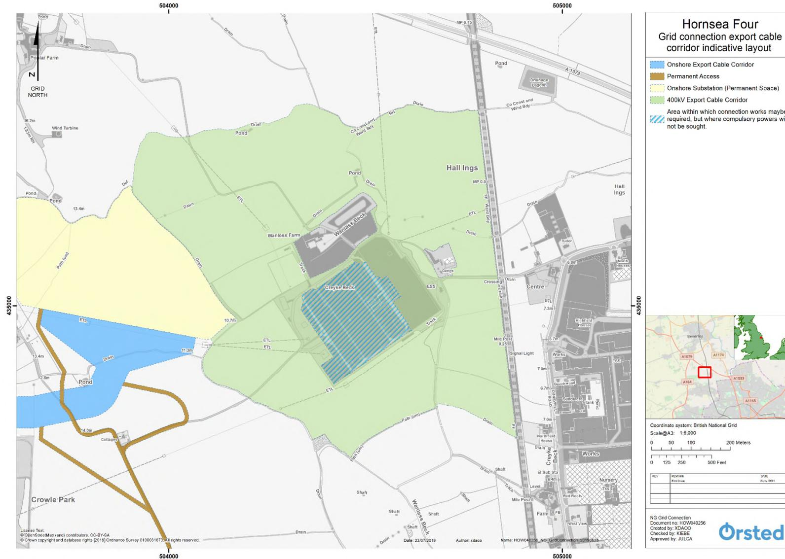
Figure 4.23: Grid connection export cable corridor indicative layout (not to scale).
