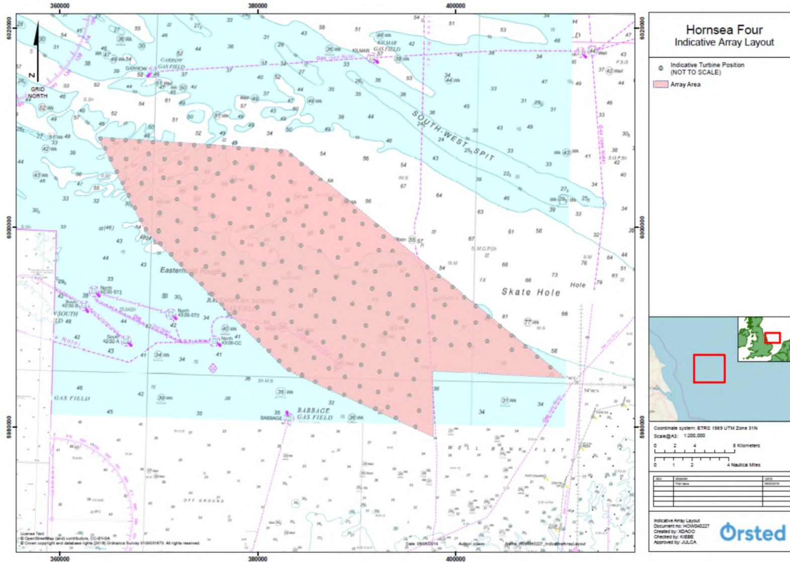
Figure 4.12: Hornsea Four Indicative layout with 190 positions. (180 WTGs, 9 substations and 1 offshore accommodation platform) (not to scale).
