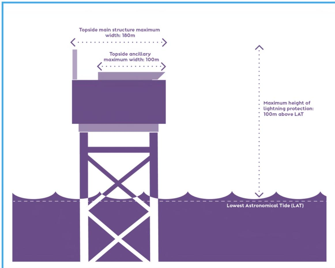
Figure 4.7: Schematic of an offshore transformer substation (indicative only).
