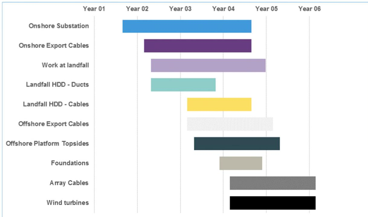
Figure 4.4: Indicative construction programme for Hornsea Four.
